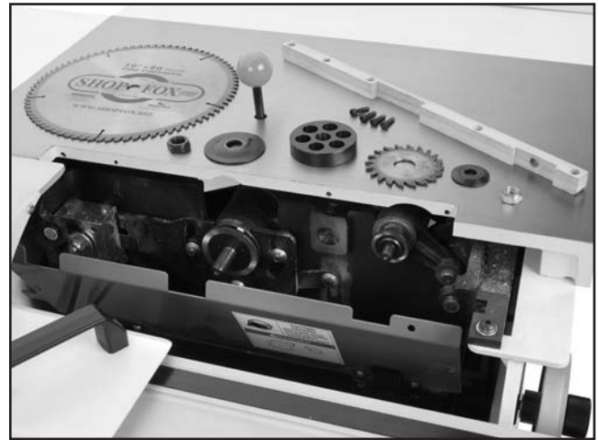
Figure 92. Original table insert and all necessary components removed.
